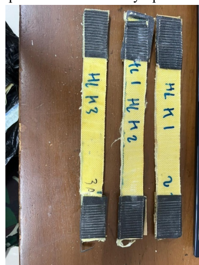
Gambar 4.26 Kevlar Hand Lay-up
