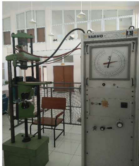
Gambar 4.14 Mesin Uji Bending Universal Bending Machine
