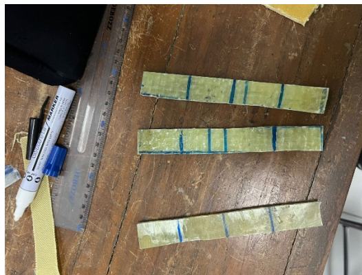
Gambar 4.18 Benda Uji 3 Fiberglass Metode Hand Lay-up
