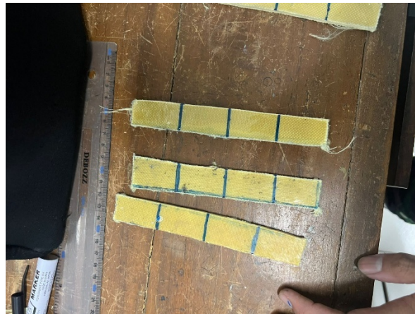
Gambar 4.19 Benda Uji 4 Kevlar Metode Hand Lay-up
