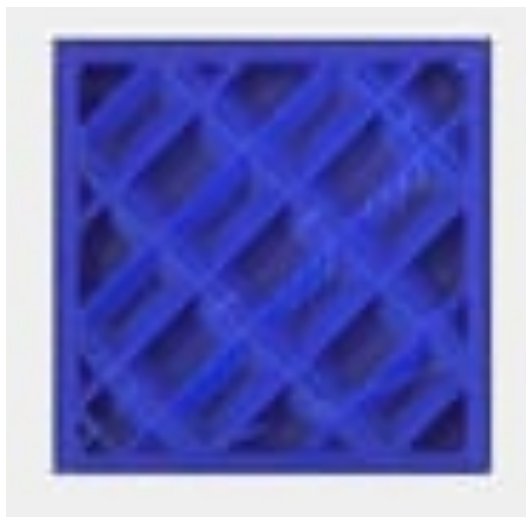
Gambar 3. Infill Pattern Quarter Cubic
